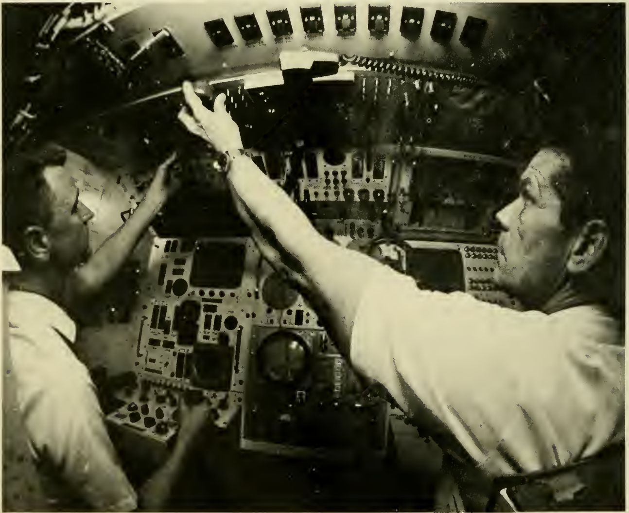
Fig. 13.3 Control console of DEEP QUEST . (LMSC)
