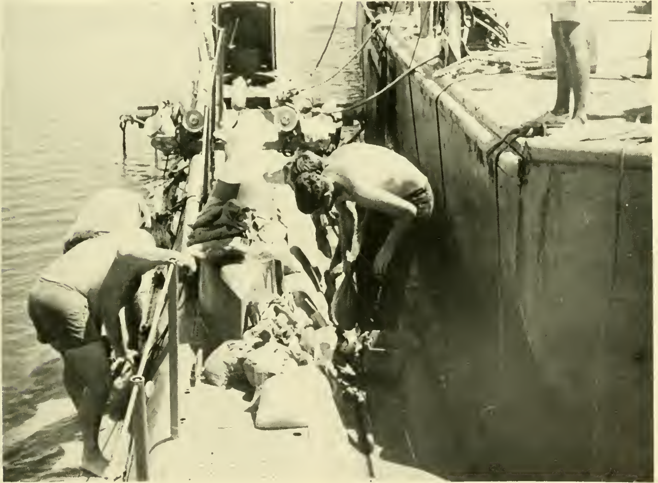
Fig 6.8 ALUMINAUT's crew loading shot ballast at Roosevelt Roads, Puerto Rico. (NAVOCEANO)
