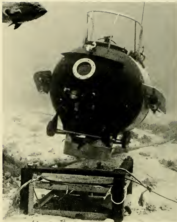
Fig. 3.11 General Dynamics' STAR I simulates rescue of personnel at 192 feet off Bermuda. (Gen. Dyn. Corp.)
