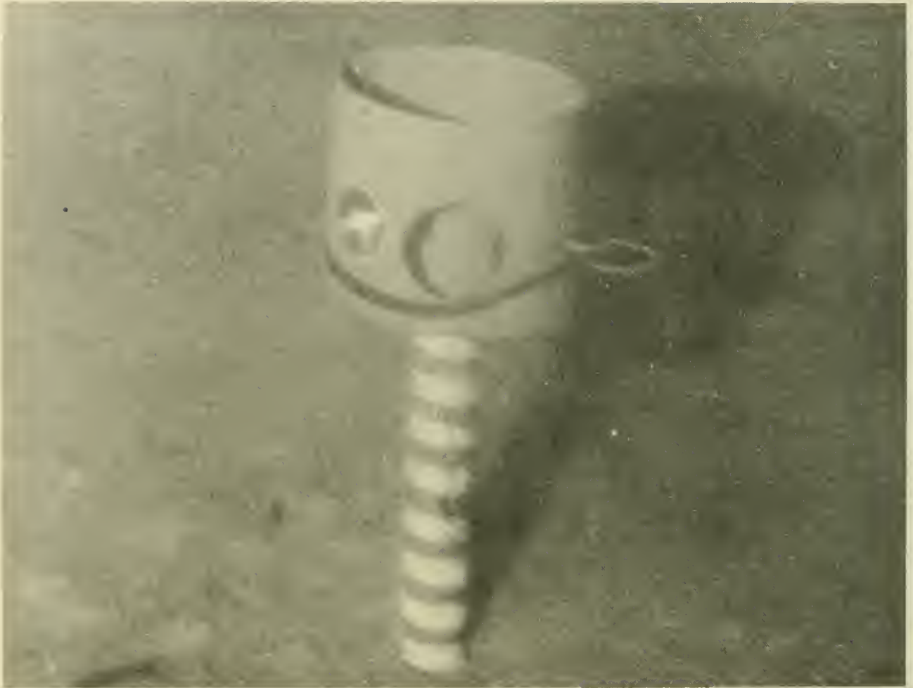
Fig. 11.18 a) A sediment strength measuring probe deployed by ALUMINAUT at 6,000 ft. The rings provide depth of penetration data and an accelerometer within a glass sphere inside the cylindrical housing provides supporting information. The glass sphere is retrieved by retracting the pin on the right which allows the sphere to surface. (NAVOCEANO) b) STAR III 's parabolic acoustic reflector transducer system was used to monitor reverberation of deep scattering layers. It also includes a stereo camera system. (Gen. Dyn.) c) A diver adjusts an apparatus on ALUMINAUT which was used in an experiment to measure sediment consolidation. When ALUMINAUT 's manipulator retracted one of the rings, a steel ball of known dimensions and density fell to the bottom, a camera photographed the sediment cloud produced and subsequently, the imbedded ball itself. (NAVOCEANO) d) A close-up of the reversing thermometer racks shown in Fig. 11.17 The solenoids (left) released the thermometer rack from its upright position when activated. (WHOI)
