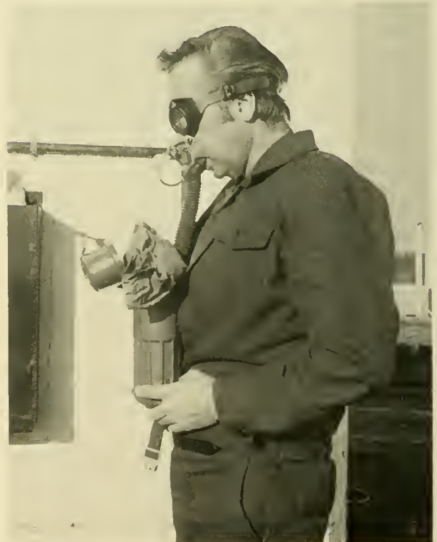
Fig 14.10 The Westinghouse Min-O'Lung (left) and Drager (right) emergency breathing systems. Both have about 0.5 hours endurance. (Westinghouse Corp.)
